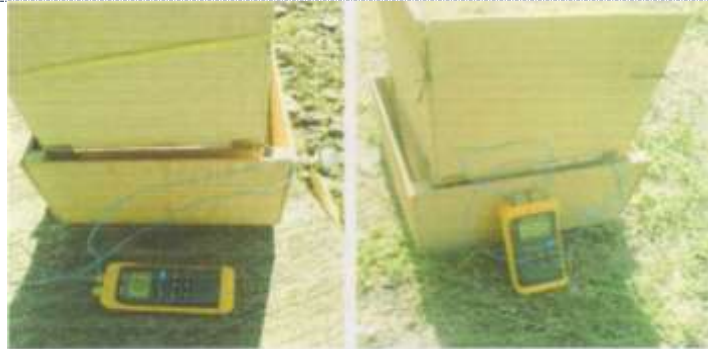
Temperature measurement at various parts of the solar box heater using digital thermometer
